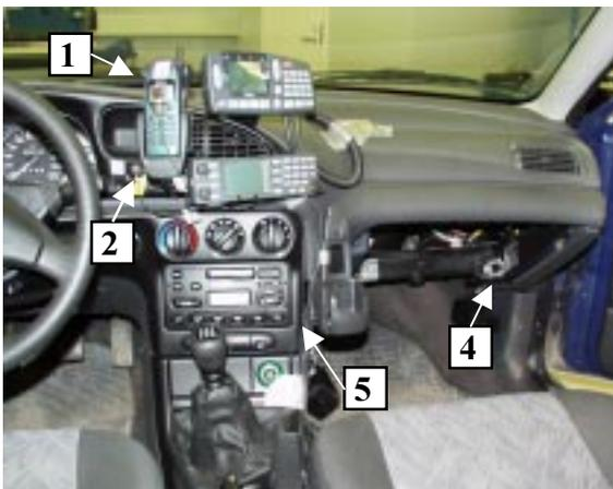
**Figure 3.** Acceleration measurement points 1,2,4 and 5.
