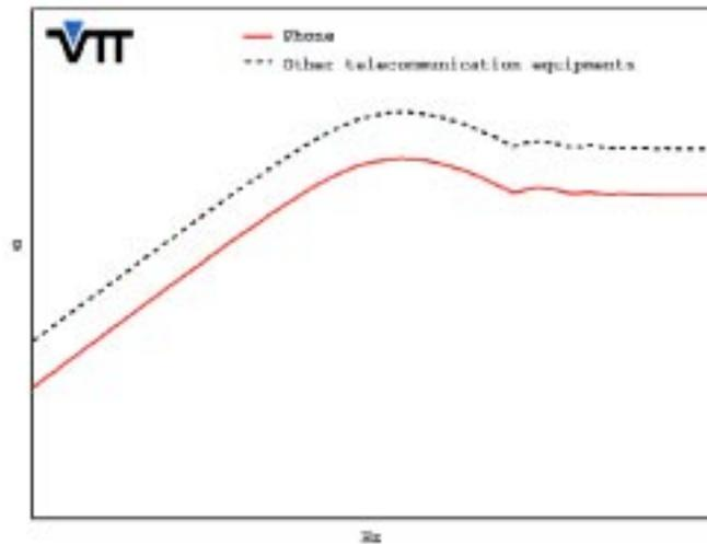
**Figure 13.** Test SRS for mobile phone and other telecommunication equipment.
