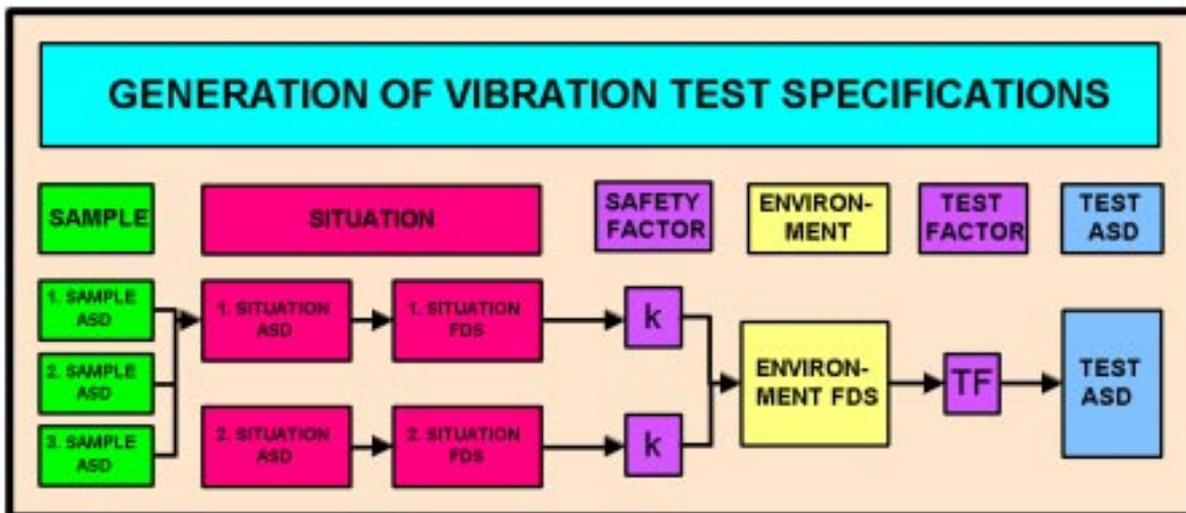
**Figure 11.** Generation of vibration test specifications.
