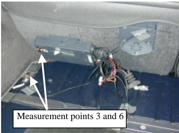
**Figure 7.** Acceleration measurement points on the back chassis of the car and on the radio unit.
