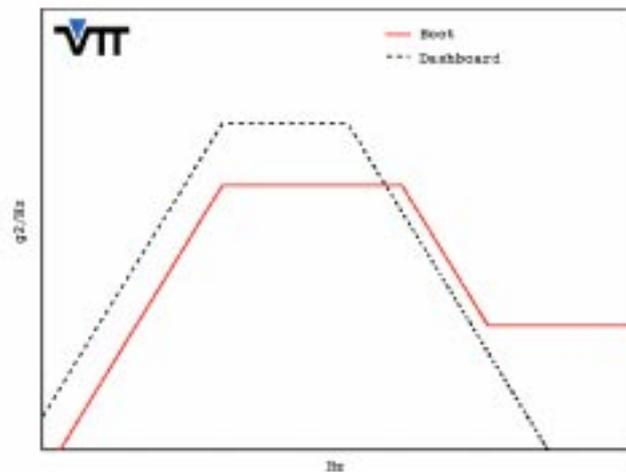
**Figure 12.** Vibration test spectra for products installed on boot and dashboard.
