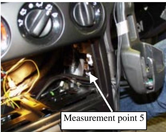
**Figure 6.** Accelerometer mounted near the car radio.
