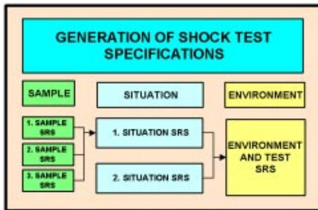
**Figure 10.** Diagram of generation of shock test specifications.
