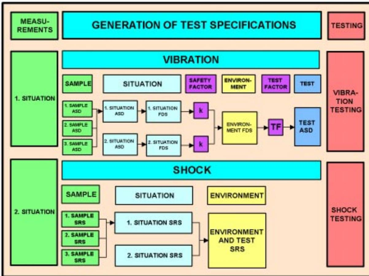
**Figure 1.** Environmental test tailoring process for shocks and vibrations.
