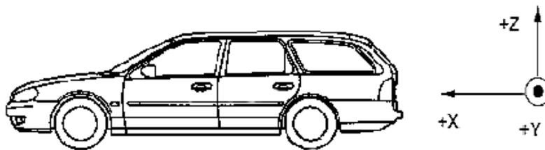
**Figure 9.** Global co-ordinate axes of vehicle.
