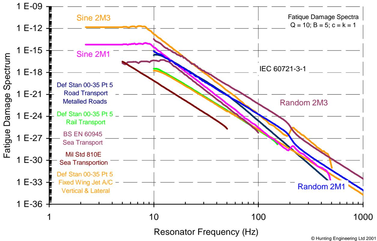
Figure 9 Comparison of IEC 60721-2 Severities with Specific Tests - FDS
