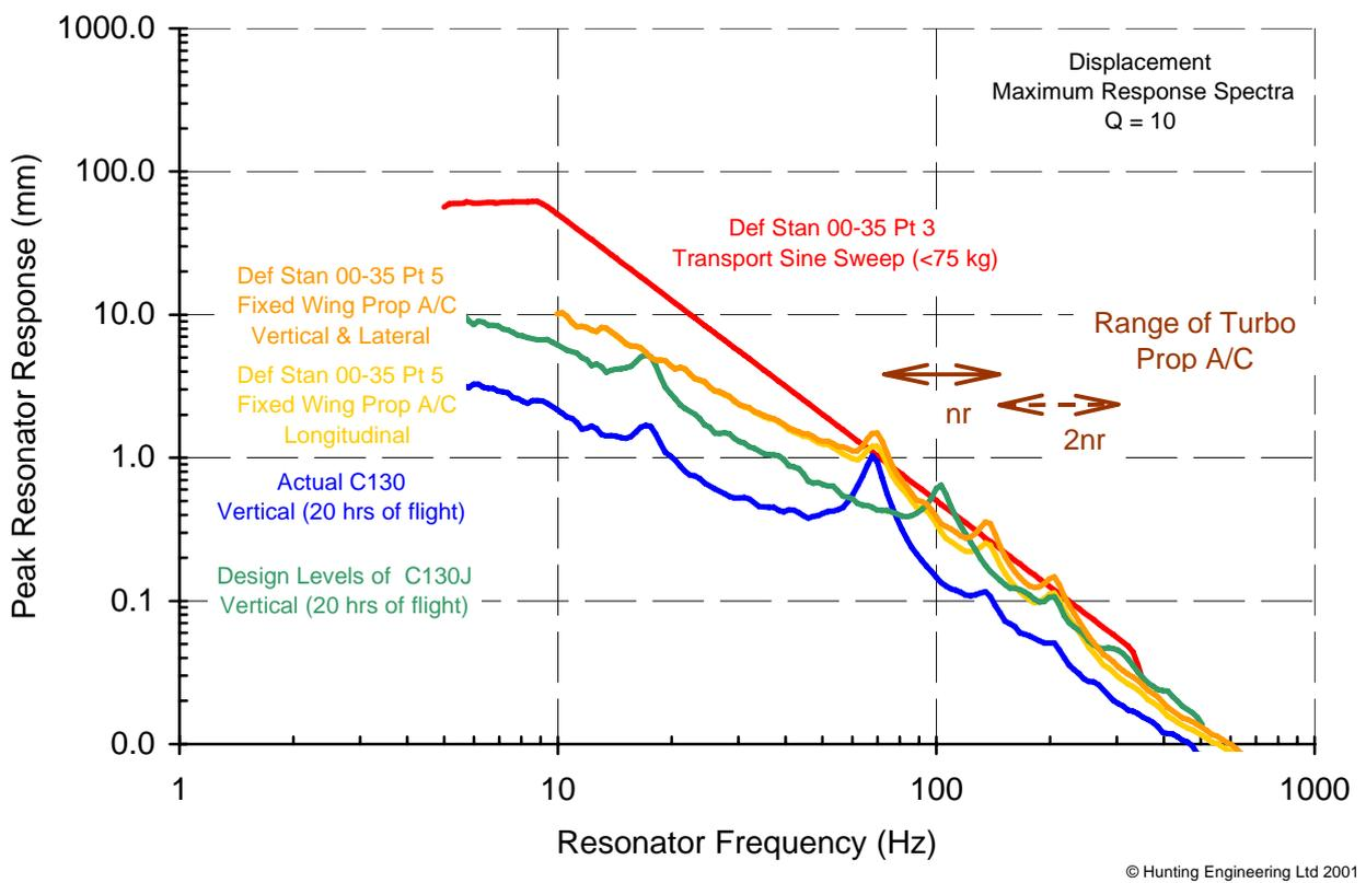
Figure 14 Comparison of Def Stan 00-35 Tests Fixed Wing Propeller Air Transportation - DMRS
