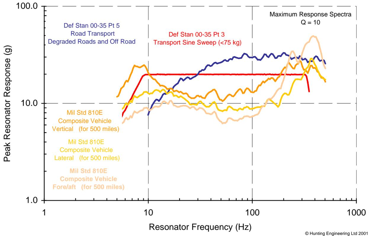
Figure 19 Comparison of Def Stan 00-35 Tests With Mil Std 810F for Wheeled Vehicle Transportation - MRS
