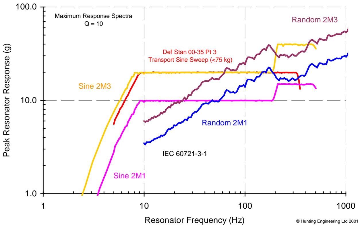
Figure 4 Comparison of Def Stan 00-35 Test and IEC 60721-3-2 Severities - MRS
