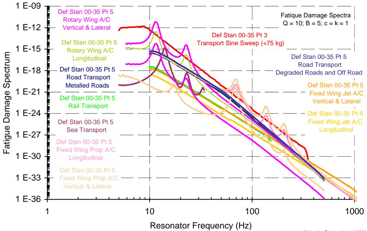
Figure 27 Comparison of Def Stan 00-35 Tests - FDS
