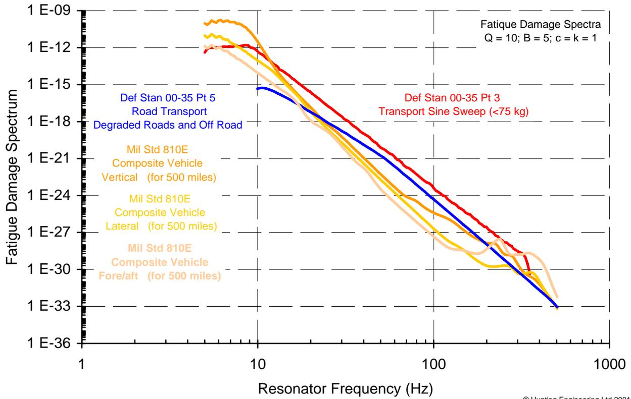
Figure 21 Comparison of Def Stan 00-35 Tests With Mil Std 810E for Wheeled Vehicle Transportation - FDS
