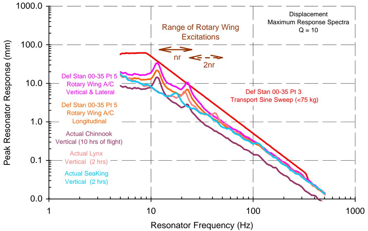
Figure 11 Comparison of Def Stan 00-35 Tests Rotary Wing Air Transportation - DMRS
