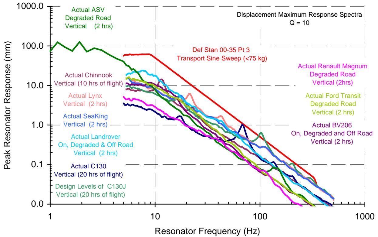
Figure 29 Comparison of Def Stan 00-35 Test With Actual Conditions - DMRS
