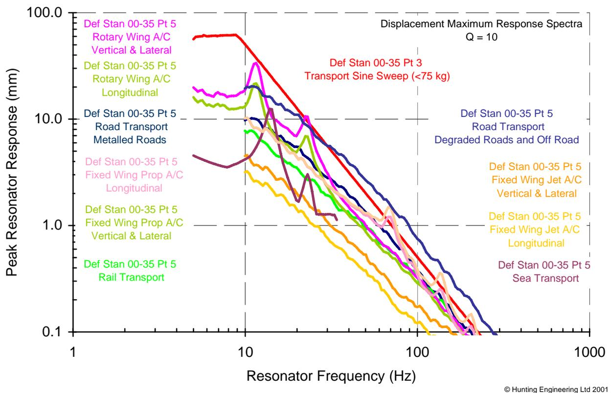
Figure 26 Comparison of Def Stan 00-35 Tests - DMRS
