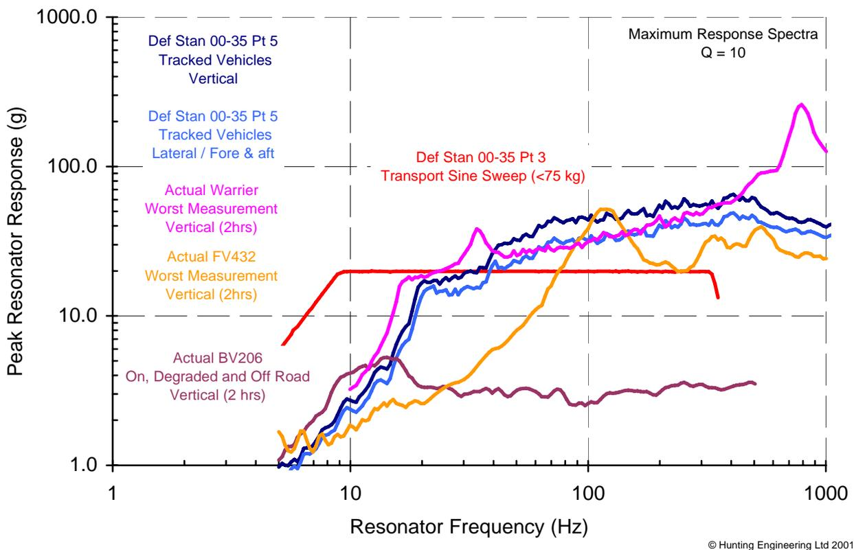
Figure 22 Comparison of Def Stan 00-35 Tests Typical 2nd to 1st Line Tracked Vehicle Transportation - MRS
