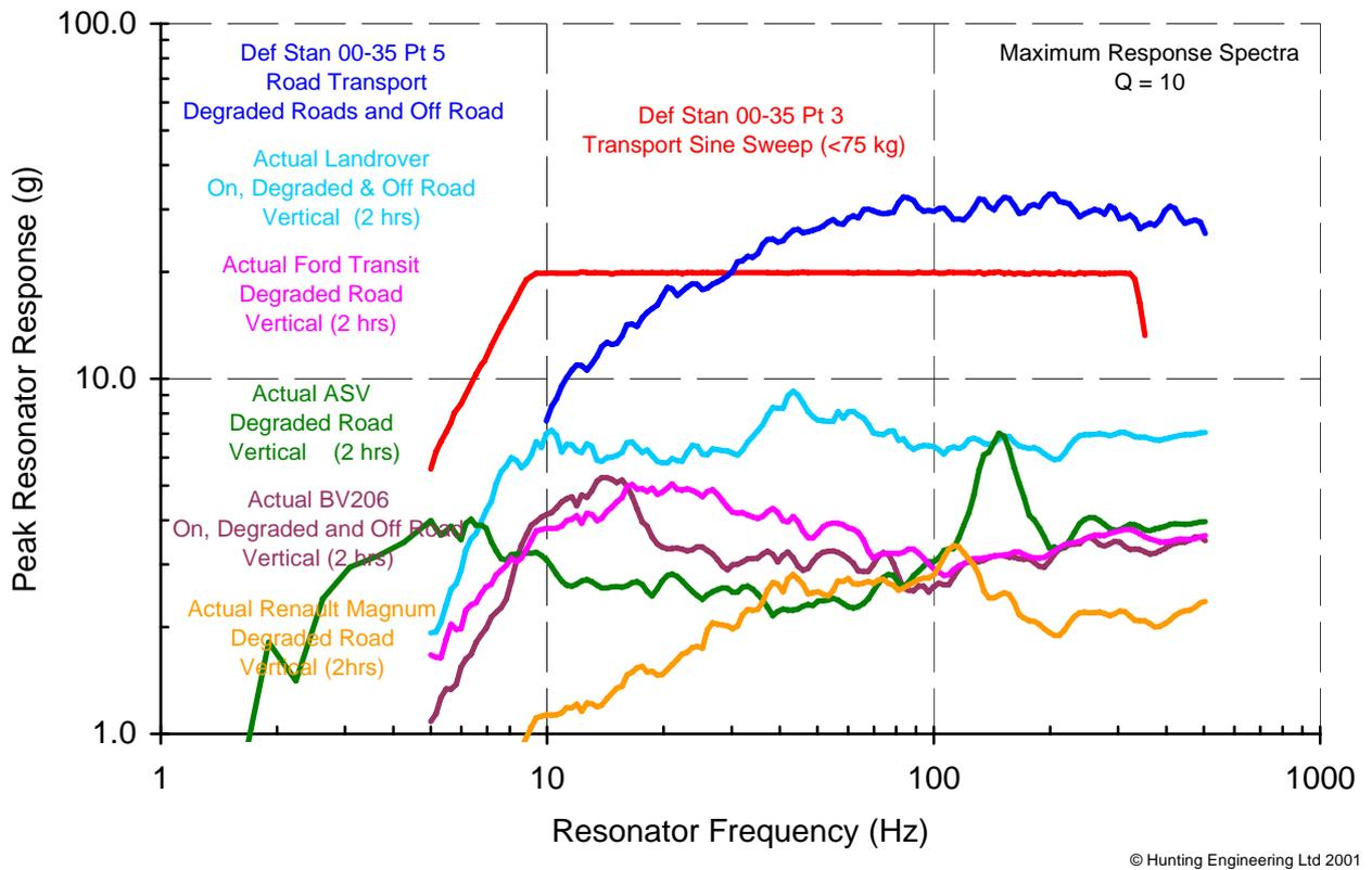
Figure 16 Comparison of Def Stan 00-35 Tests Typical 2nd to 1st Line Wheeled Vehicle Transportation - MRS
