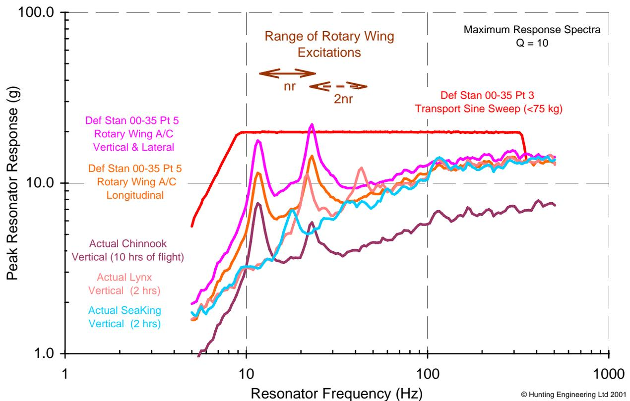
Figure 10 Comparison of Def Stan 00-35 Tests Rotary Wing Air Transportation - MRS
