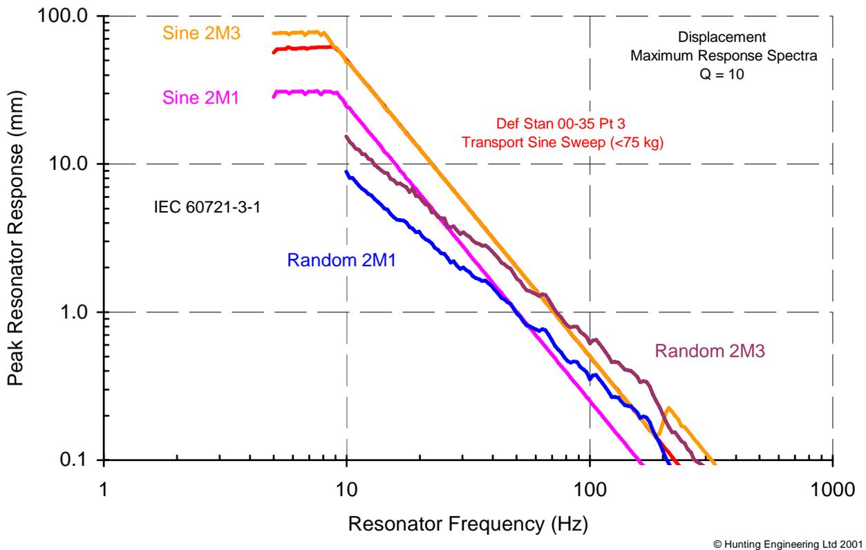
Figure 6 Comparison of Def Stan 00-35 Test and IEC 60721-3-2 Severities - DMRS
