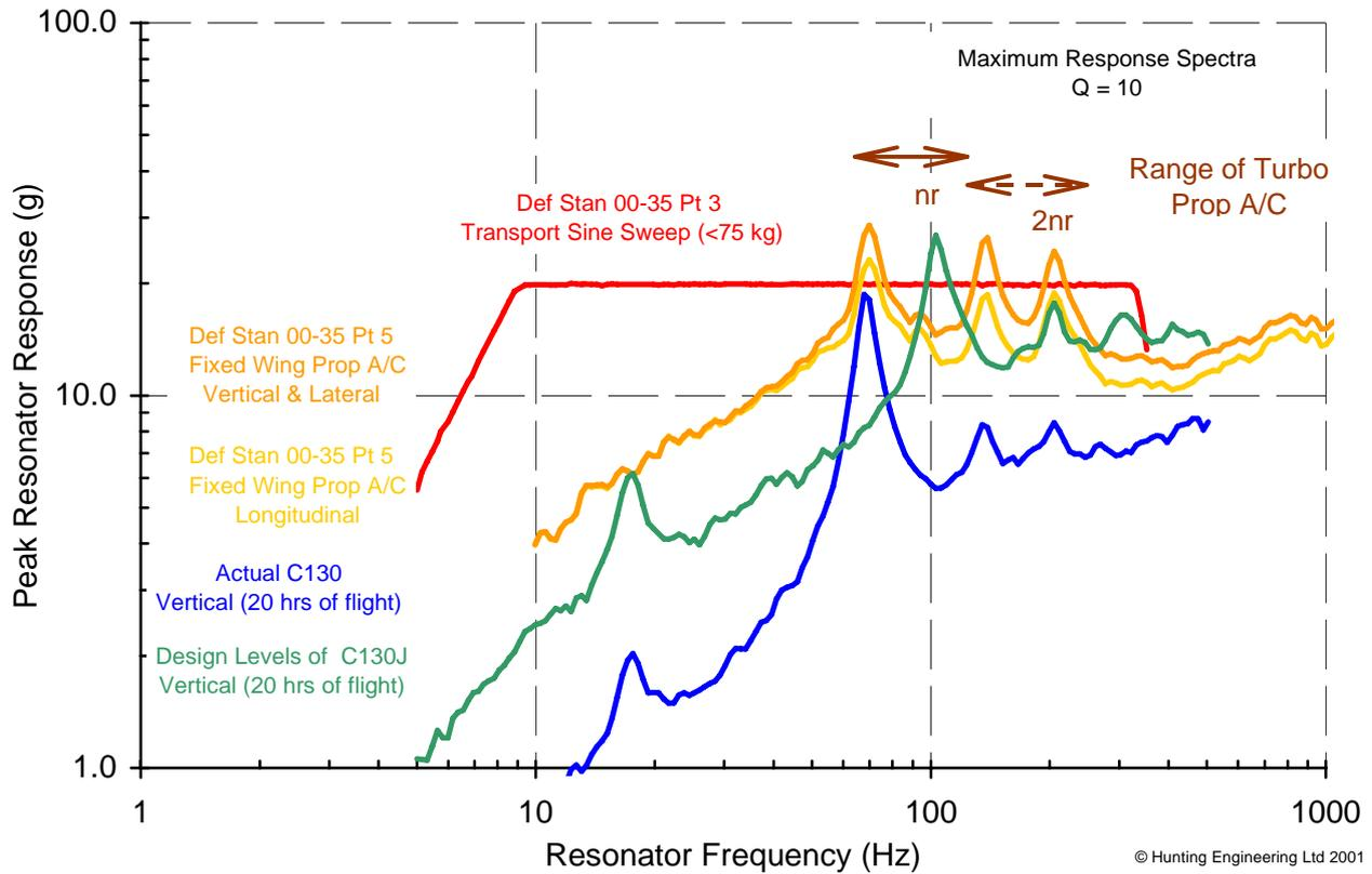
Figure 13 Comparison of Def Stan 00-35 Tests Fixed Wing Propeller Air Transportation - MRS
