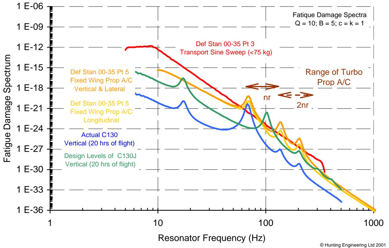
Figure 15 Comparison of Def Stan 00-35 Tests Fixed Wing Propeller Air Transportation - FDS
