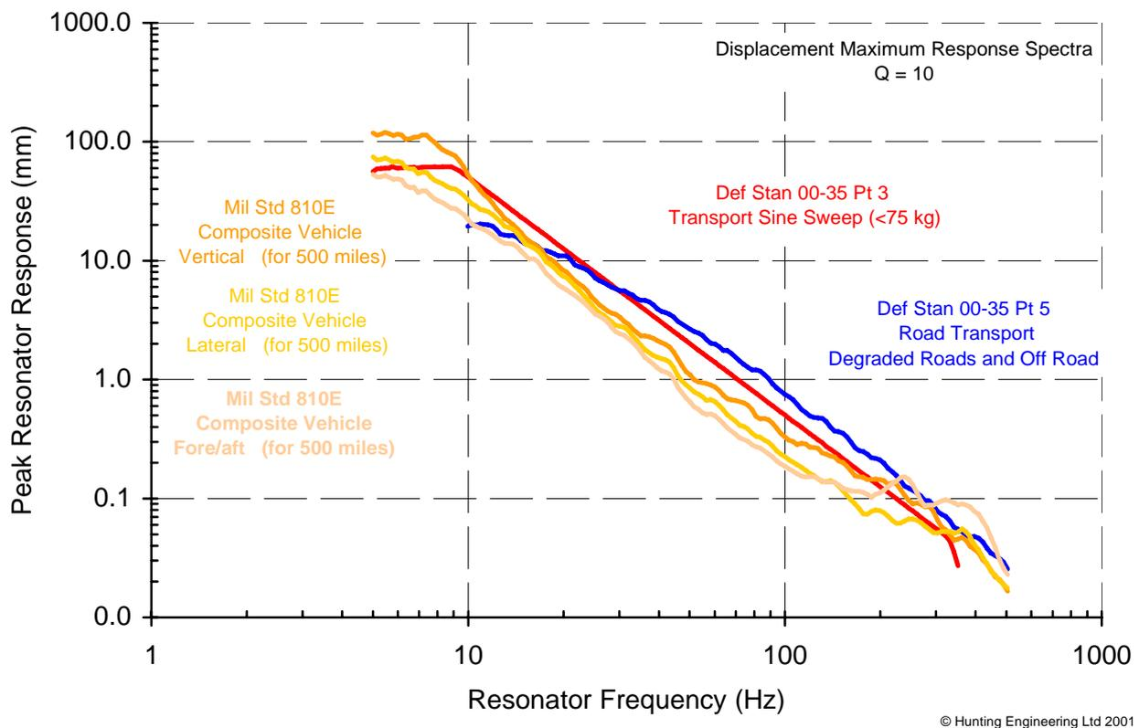
Figure 20 Comparison of Def Stan 00-35 Tests With Mil Std 810F for Wheeled Vehicle Transportation - DMRS
