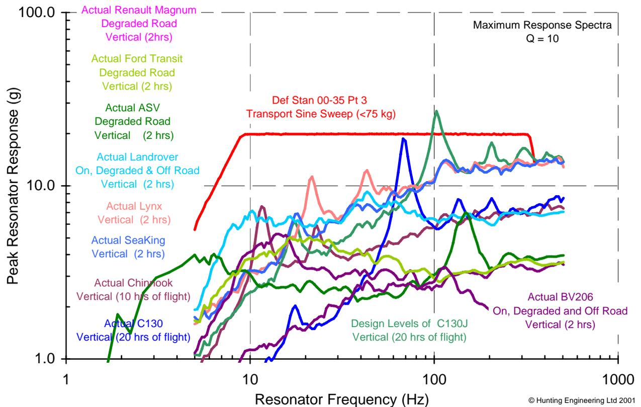
Figure 28 Comparison of Def Stan 00-35 Test With Actual Conditions - MRS
