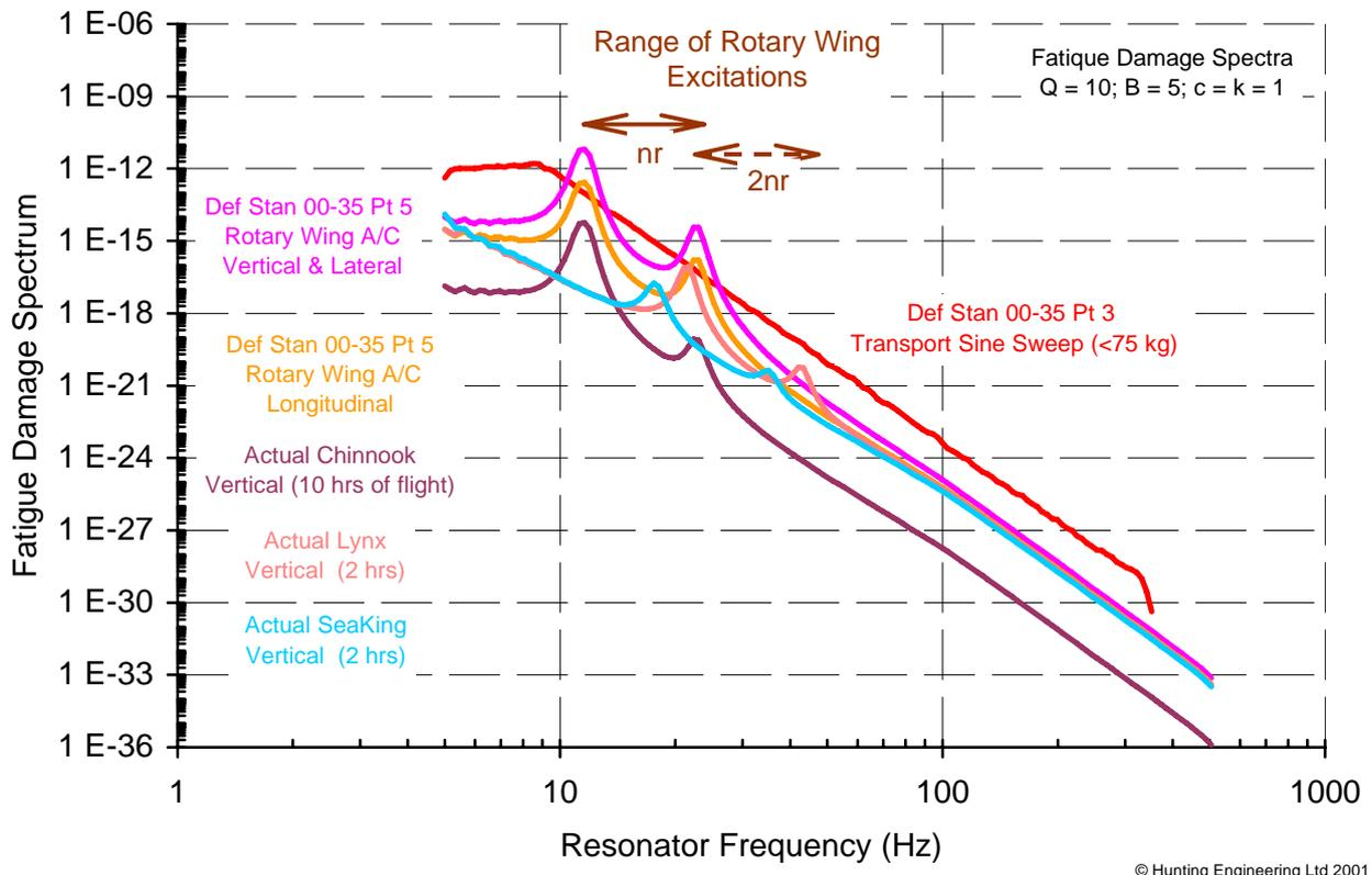
Figure 12 Comparison of Def Stan 00-35 Tests Rotary Wing Air Transportation - FDS
