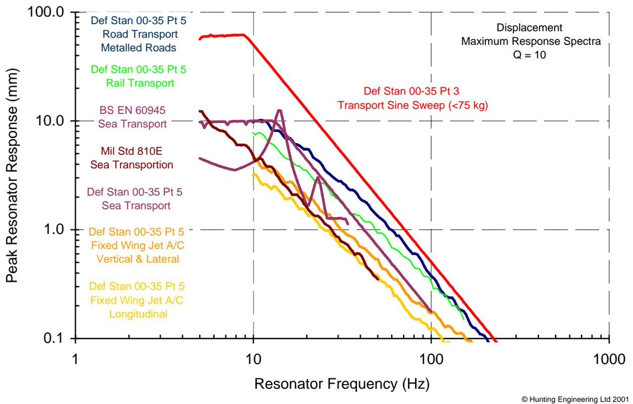
Figure 2 Comparison of Def Stan 00-35 Tests Typical 3rd to 2nd Line Transportation - DMRS
