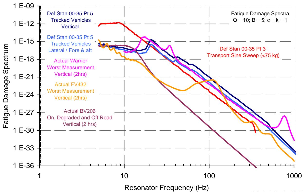
Figure 24 Comparison of Def Stan 00-35 Tests Typical 2nd to 1st Line Tracked Vehicle Transportation - FDS
