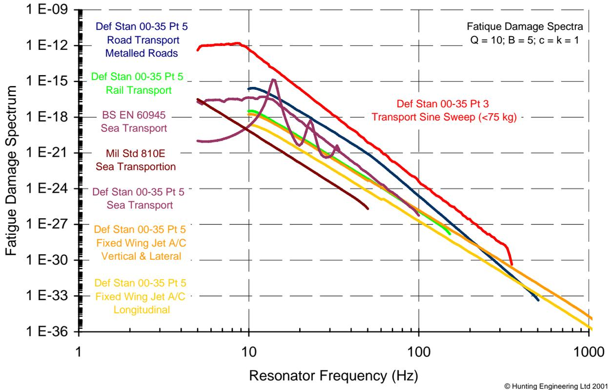
Figure 3 Comparison of Def Stan 00-35 Tests Typical 3rd to 2nd Line Transportation - FDS
