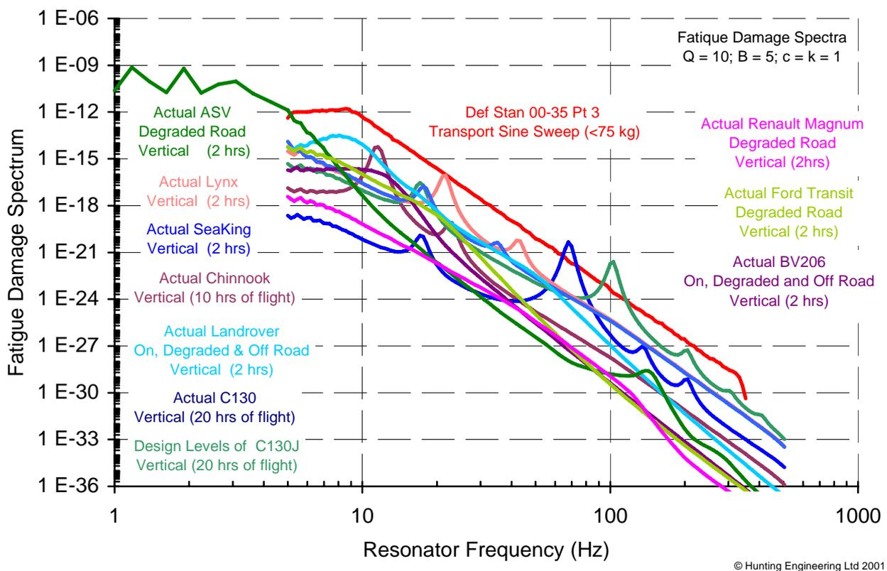
Figure 30 Comparison of Def Stan 00-35 Test With Actual Conditions - FDS
