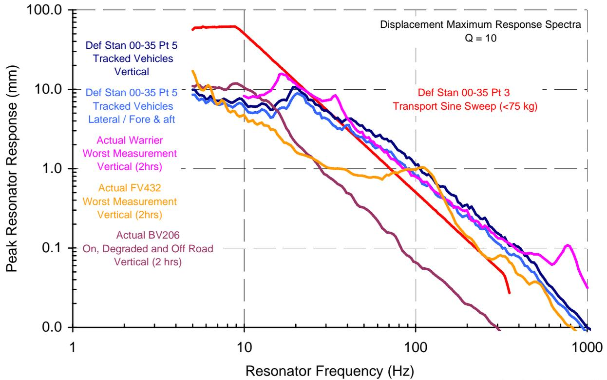
Figure 23 Comparison of Def Stan 00-35 Tests Typical 2nd to 1st Line Tracked Vehicle Transportation - DMRS
