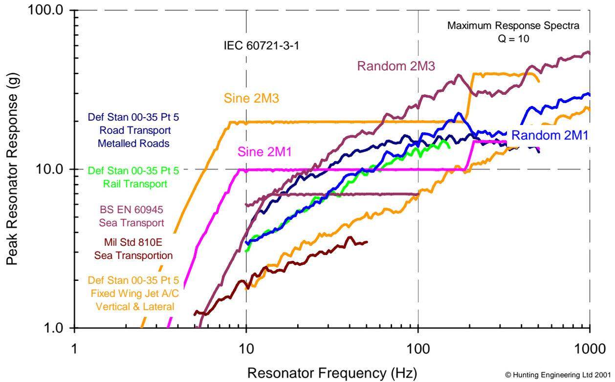
Figure 5 Comparison of IEC 60721-3-2 Severities with Specific Tests - MRS
