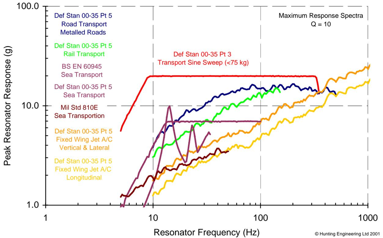
Figure 1 Comparison of Def Stan 00-35 Tests Typical 3rd to 2nd Line Transportation - MRS
